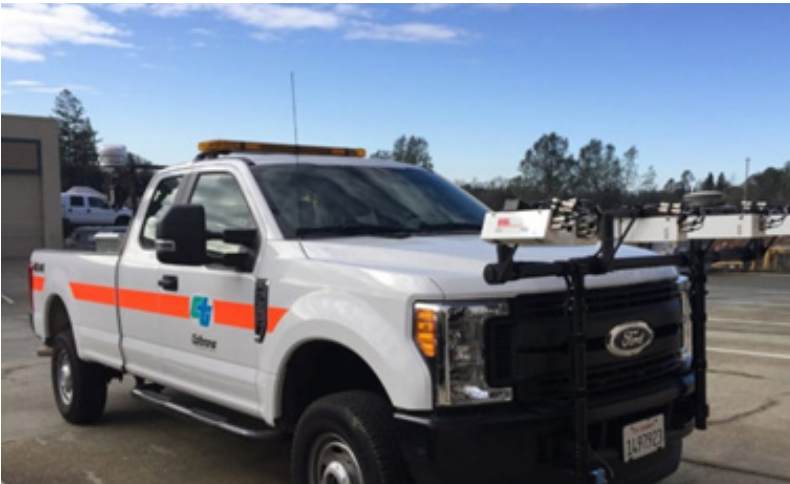
Truck Mounted Camera System for PCI Measurement
